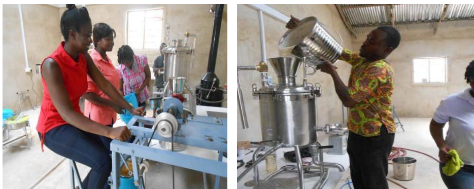
A SARI technician pedals a bicycle operated grinder at the SoyCow facility, while another technician adds ground soybeans to the cookers to produce soy milk.
