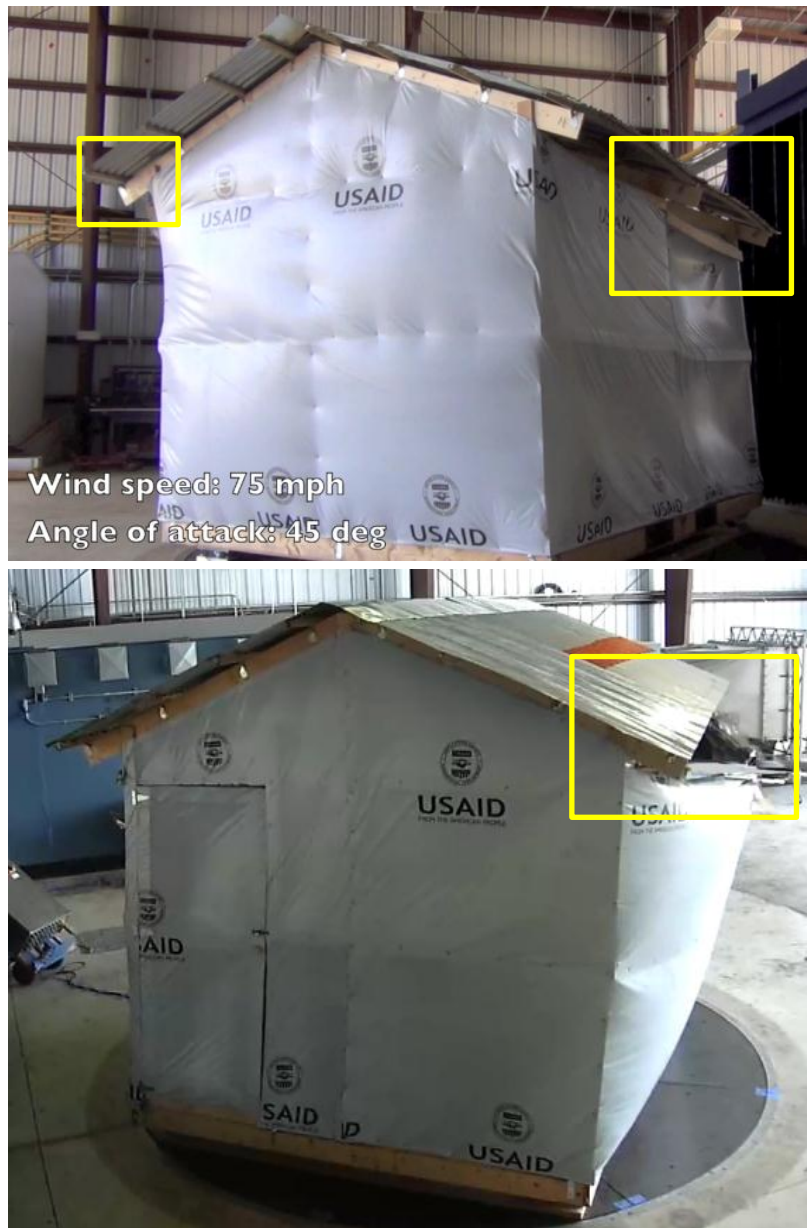
Figure 23 - Test at 75 mph and 45°; horizontal members detaching from framing
