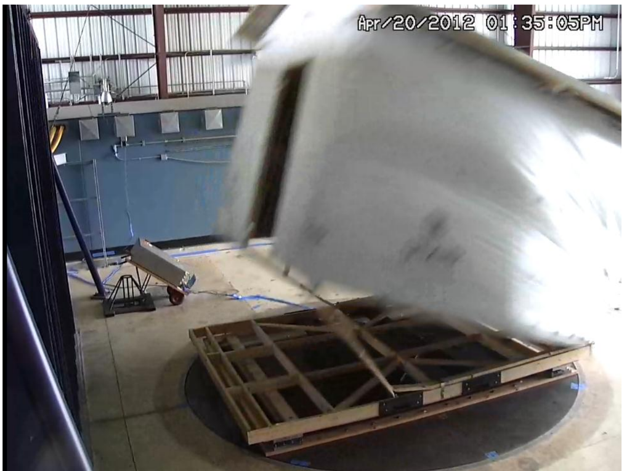
Figure 29 - Platform base failure due to increased uplift tension on wood members
