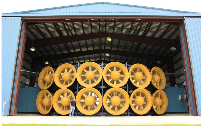
Figure 1 – Testing equipment: Twelve-fan Wall of Wind
