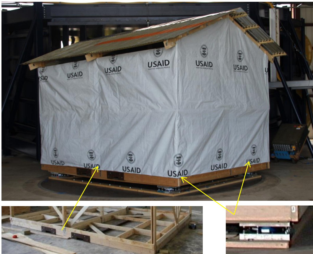
Figure 20 - Base platform and load cell for T-Shelter tests
