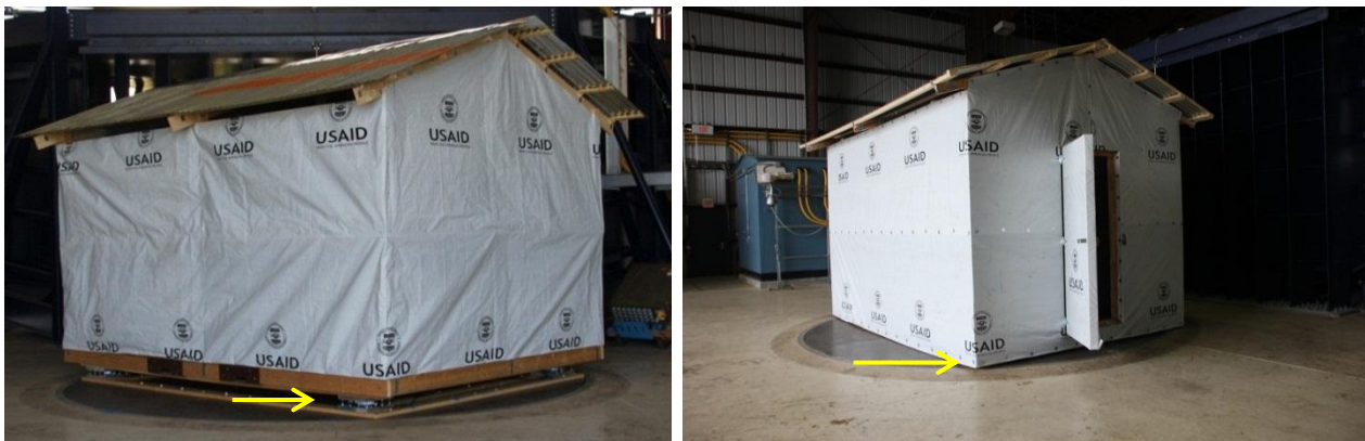
Figure 2 - Base platform and load cell for T-Shelter tests. Arrows point out the difference: with and without 6-DOF load cells
