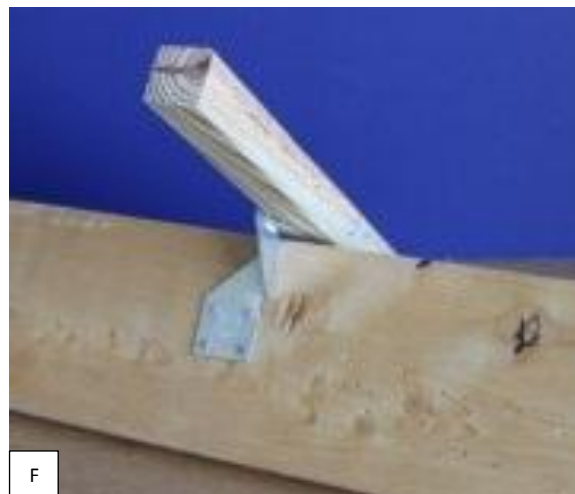
Figure 17 – Hurricane strapping techniques: (A) metal straps on 2-inx4-in, (B) metal strap on 2-inx2-in and 1-inx6-in, (C) metal wire on 2-inx4-in, (D) metal wire on 2-inx2-in and 2-inx4-in, (E) engineered tie on 2-inx4-in and (F) engineered tie on 2-inx2-in and 1-inx6-in
