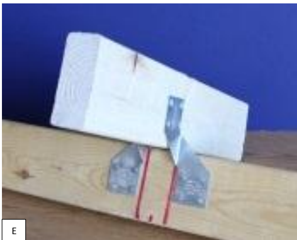
Figure 17 – Hurricane strapping techniques: (A) metal straps on 2-inx4-in, (B) metal strap on 2-inx2-in and 1-inx6-in, (C) metal wire on 2-inx4-in, (D) metal wire on 2-inx2-in and 2-inx4-in, (E) engineered tie on 2-inx4-in and (F) engineered tie on 2-inx2-in and 1-inx6-in
