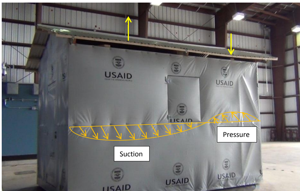
Figure 5 - T-Shelter 3 test at 85 mph and 90° angle of attack
