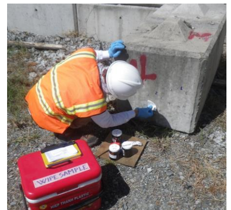
Collecting a wipe sample from the surface of the treatment structure wall (Photo: CDM Smith)
