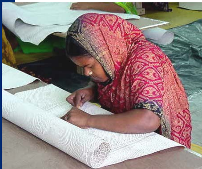
A Bangladeshi woman embosses leather that will be used to manufacture handbags and shoes for export.
