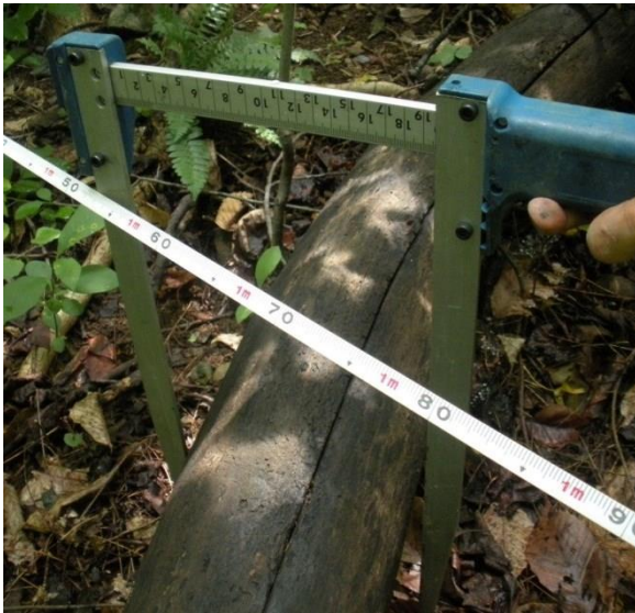
Figure 10: Use of calipers to measure the diameter of lying deadwood
