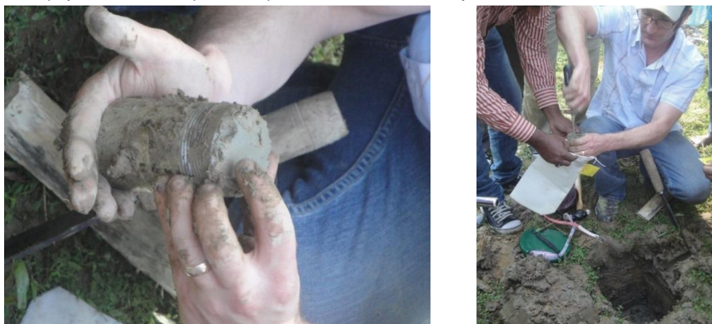
Figure 14: Bulk density ring with soil samples; and the pit from where soil profile is taken.
